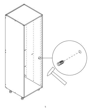
Knock in the bushings to your desired height by using a hammer. Do not install the doors before the shelf is in place. Consider hinge placement when planning the location of your shelf.
