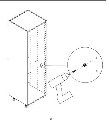
Fasten the screw through the plastic sleeve.
