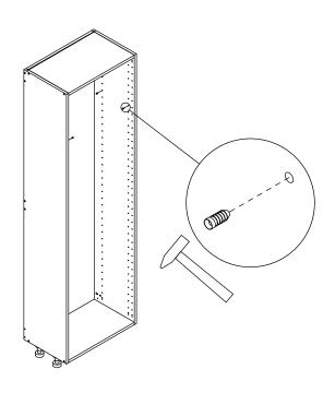
$\label{eq:continuous} \begin{tabular}{ll} $\delta$ \\ Knock in the bushings to your desired height by using a hammer . \\ \end{tabular}$
