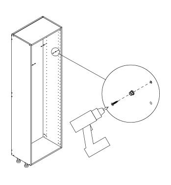
Fasten the screw through the plastic sleeve.
