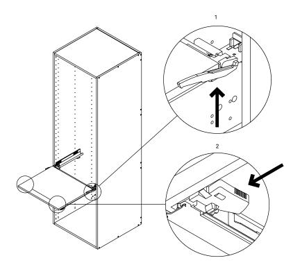
To remove your shelf, lift the lock while drawer slides are extended and press on the two orange levers simultaneously to lift it up.
