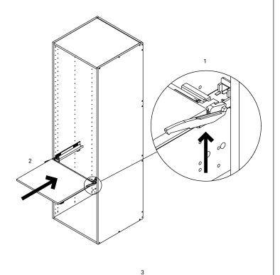
Place the shelf onto the open drawer slides, lift the lock in the back and slide it in.
