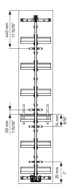
Plan the location of your brackets. If the suggested placement of your brackets interferes with your desired shelf location, move the brackets to another position.
