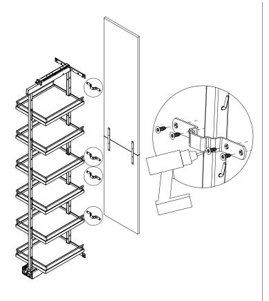
Fasten the brackets onto the front using the included screws.
