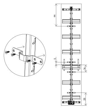
FASTEN THE BRACKETS ONTO THE FRONT USING THE INCLUDED SCREWS. YOU CAN USE THE MEASUREMENTS ON THE DRAWING AS A GUIDELINE—ALTHOUGH THEY DON'T NEED TO BE PRECISE. MEASUREMENTS ARE IN CM.
