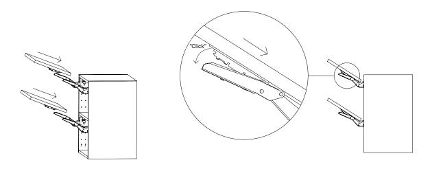
\$12\$ ALIGN THE HINGE BRACKETS ON THE FRONTS WITH THE OPEN HINGES AND PRESS THEM IN PLACE UNTIL YOU HEAR A CLICK.
