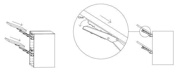
12 ALIGN THE HINGE BRACKETS ON THE FRONTS WITH THE OPEN HINGES AND PRESS THEM IN PLACE UNTIL YOU HEAR A CLICK.
