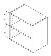
2 INSERT SHELF HOLDERS INTO THE PRE-DRILLED HOLES INSIDE THE CABINET AND INSTALL THE SHELF. MAKE SURE TO USE THE HOLES THAT ARE EXACTLY MID-HEIGHT OF THE CABINET.
