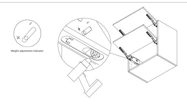
FOR THE HINGES TO OPEN PROPERLY, THE HINGES NEED TO BE ADJUSTED TO THE WEIGHT OF THE FRONTS.
