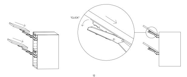
ALIGN THE HINGE BRACKETS ON THE FRONTS WITH THE OPEN HINGES AND PRESS THEM IN PLACE UNTIL YOU HEAR A CLICK.
