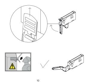
WHILE PUSHING UP ON THE ORANGE PLASTIC PIECE, PULL OUT THE HINGE MECHANISM. BE CAREFUL WHEN WORKING WITH THE HINGES, AS THE MECHANISM MAY OPEN UNEXPECTEDLY AND WITH BIG FORCE.
