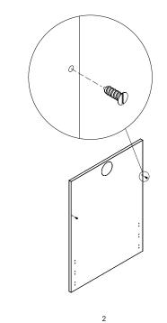
FASTEN THE WOOD SCREWS INTO THE PREDRULLED HOLES. THE SCREW HEAD MUST NOT PENERTRATE FURTHER THAN THE SURFACE OF THE DRAWER FRONT
