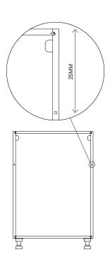
MARK THE DRILLING POSITIONS AS SHOWN ABOVE. DRILL 13MM DEEP HOLES USING A 8MM DRILL BIT. MAKE SURE THE HOLES ARE CENTERED BETWEEN THE EDGES OF THE CABINET SIDES
