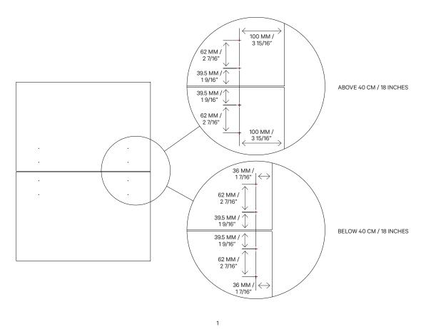
MEASURE AND MARK THE POSITION OF THE SCREWS DEPENDING ON THE WIDTH OF YOUR FRONTS.
