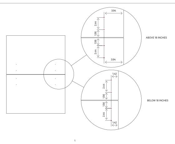
MEASURE AND MARK THE POSITION OF THE SCREWS DEPENDING ON THE WIDTH OF YOUR FRONTS. ALL DIMENSIONS ON THE ILLUSTRATION ARE IN INCHES.
