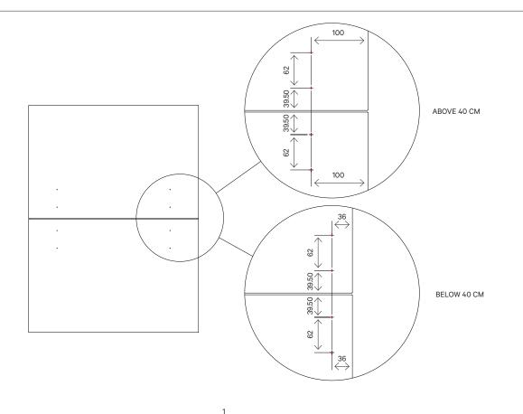
MEASURE AND MARK THE POSITION OF THE SCREWS DEPENDING ON THE WIDTH OF YOUR FRONTS. ALL DIMENSIONS ON THE ILLUSTRATION ARE IN MM.
