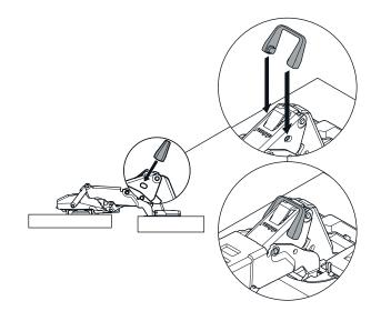
INSTALL THE ANGLE STOP BRACKET, SIMPLY BY PRESSING IT ON LIKE SHOWN ABOVE.
