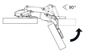
FOR ALL DOORS WITH A THICKNESS ABOVE 21MM, YOU NEED TO LIMIT THE OPENING ANGLE OF THE 155 DEGREE HINGES TO 90 DEGREES USING THE INCLUDED ANGLE-STOP BRACKET
