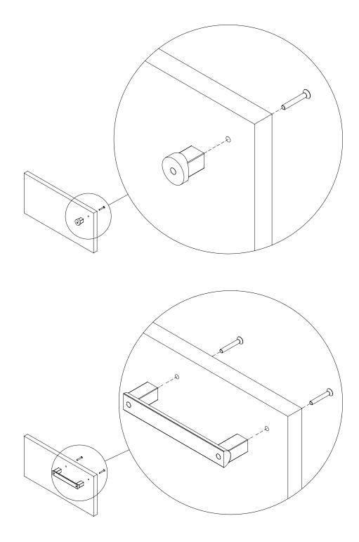
FASTEN THE HANDLE BY HAND USING A MANUAL SCREW DRIVER.
