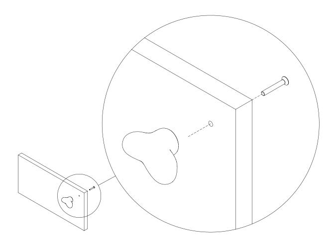
FASTEN THE HANDLE BY HAND USING A MANUAL SCREW DRIVER.
