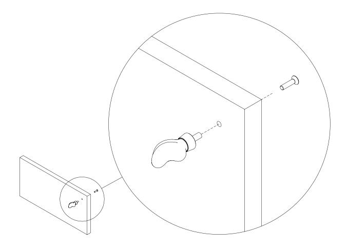
FASTEN THE HANDLE BY HAND USING A MANUAL SCREW DRIVER.
