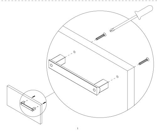
Fasten the handle by hand using a manual screw driver.
